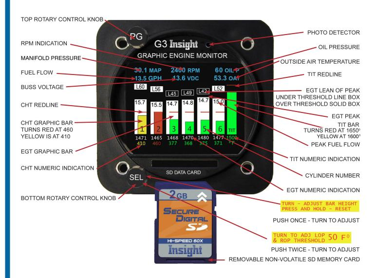
The instrument has two control knobs that operate combination rotary and push button switches. The top knob in general controls screen selection while the bottom knob controls items within the given screen.
