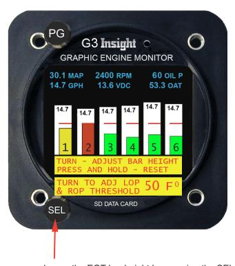
For better visibility you can change the EGT bar height by pressing the SEL knob and rotating it to set the desired height. Pressing the SEL knob a second time allows you to adjust the leaning target (set to 50 deg F below peak EGT from the factory). Press SEL a third time to save your adjustments.
