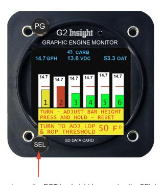
For better visibility you can change the EGT bar height by pressing the SEL knob and rotating it to set the desired height. Pressing the SEL knob a second time allows you to adjust the leaning target (set to 50 deg F below peak EGT from the factory). Press SEL a third time to save your adjustments.
