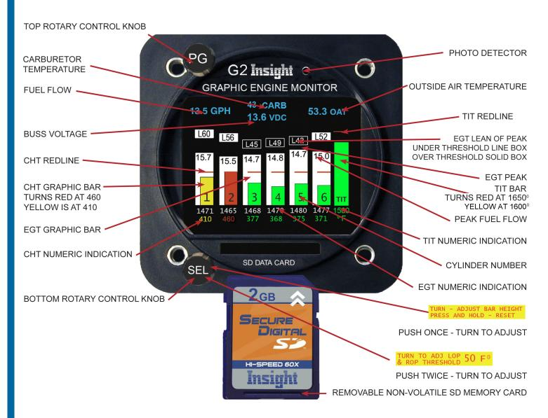
The instrument has two control knobs that operate combination rotary and push button switches. The top knob in general controls screen selection while the bottom knob controls items within the given screen.
