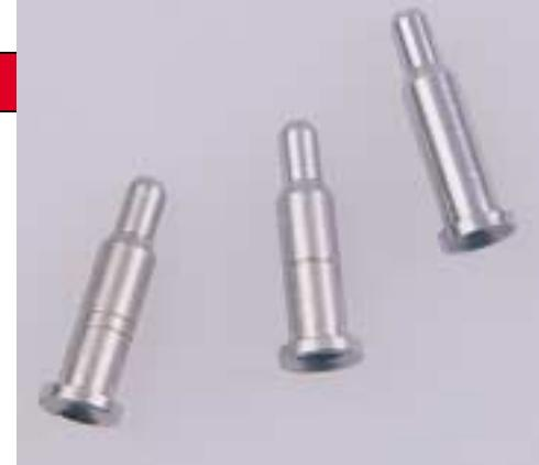
*Lycoming nozzle inserts are identified by notches around the circumference of the insert. All normally aspirated engines use the single-notch insert (also used by some turbocharged nozzles). Two-notched inserts and stepped-tube inserts (not shown) are only used on turbocharged nozzles.*
