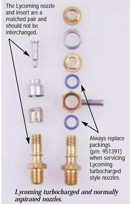
*Lycoming turbocharged and normally aspirated nozzles.*
