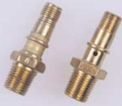
*Lycoming nozzles: The nozzle on the left must be replaced due to wear caused by a loose fitting screen shroud. Always position Lycoming nozzles with the "A" facing down and the air-bleed hole up.*
